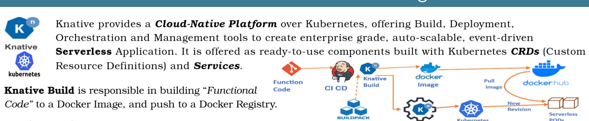
**Knative Serving** manages deployment, routing, configuration, revision and deployment of Serverless Function Containers as
